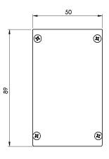
Dimensions: 1000 x 50 x 89 mm Total power:25 w Luminaire luminous flux: 2500 lm Luminaire efficacy: 100 lm/w Weight: 1.7 kg
